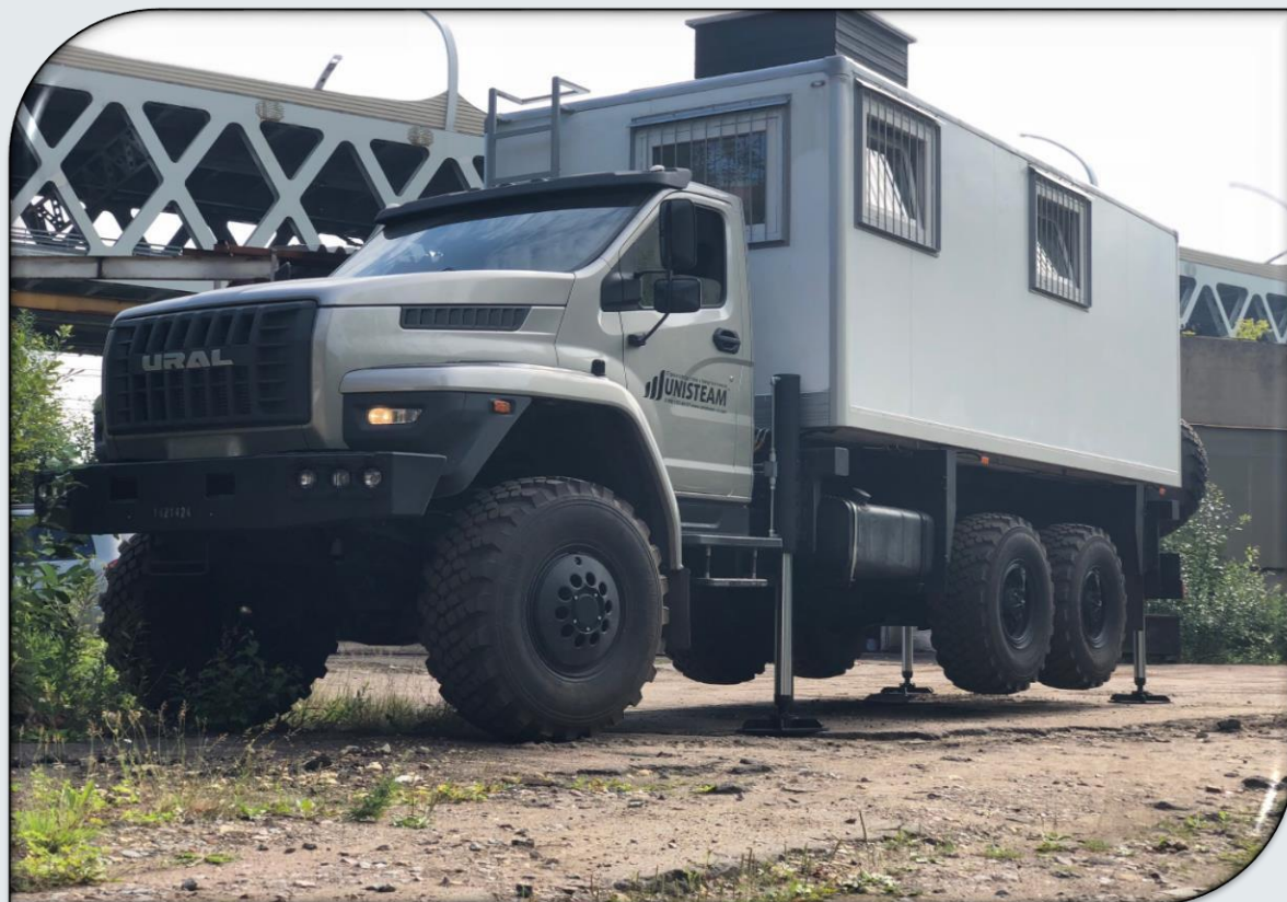
The installation of static sensing USZ-22.ZBT based on the chassis URAL NEXT
